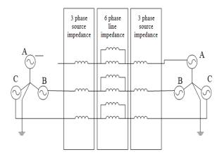
Fig. 4 Three-phase simplified system with six-phase transmission line network.
