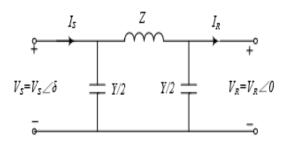
Fig.3 Equivalent  $\pi$  circuit for a lossless line
